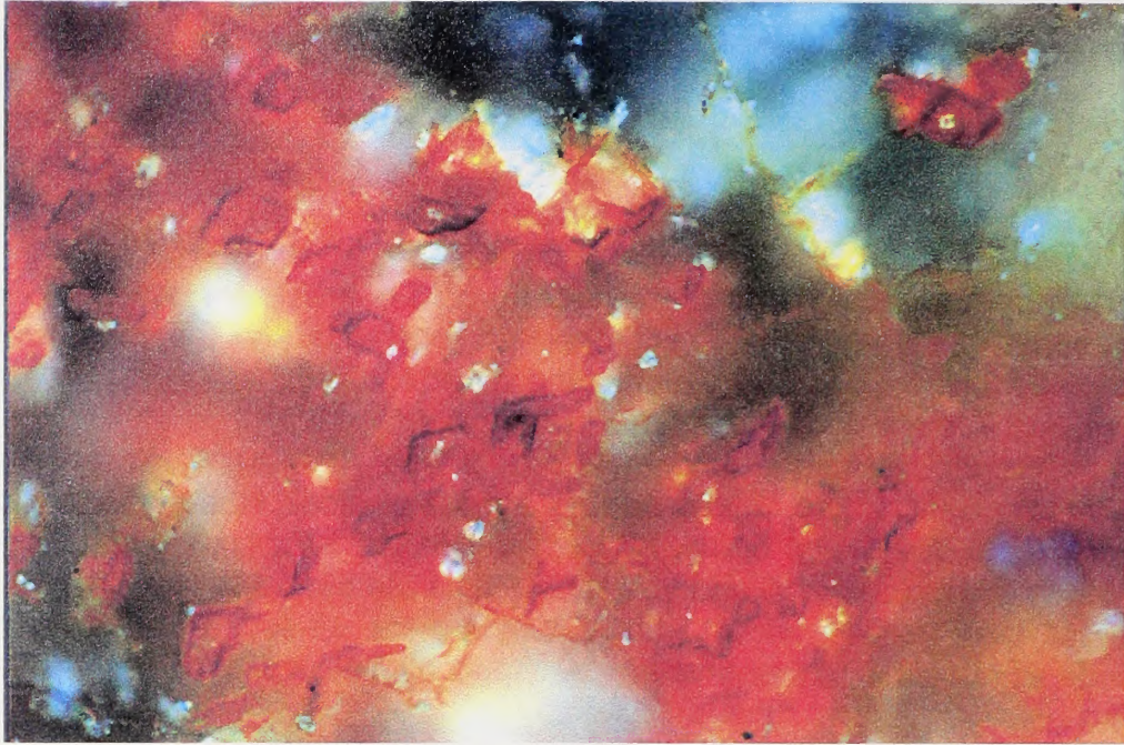
Fig.25: Photomicrograph of ironhydroxides (FeOOH) in microfractures in calcite and ankerite. Reflected light on polished surface, oil imersion, crossed-polars. Bottom edge of picture is 0.28 mm in length.
